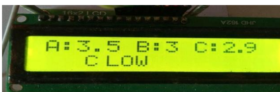
Fig 5. Low Voltage Detection in Cell-C
